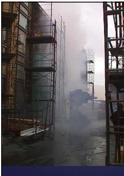
AAMA 501.1-05 Standard Test Method for Exterior Windows, Curtain Walls, and Doors for Water Penetration Using Dynamic Pressure
