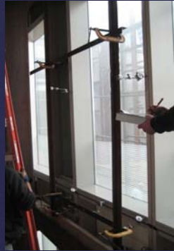
Gauges measure movement of the specimen
