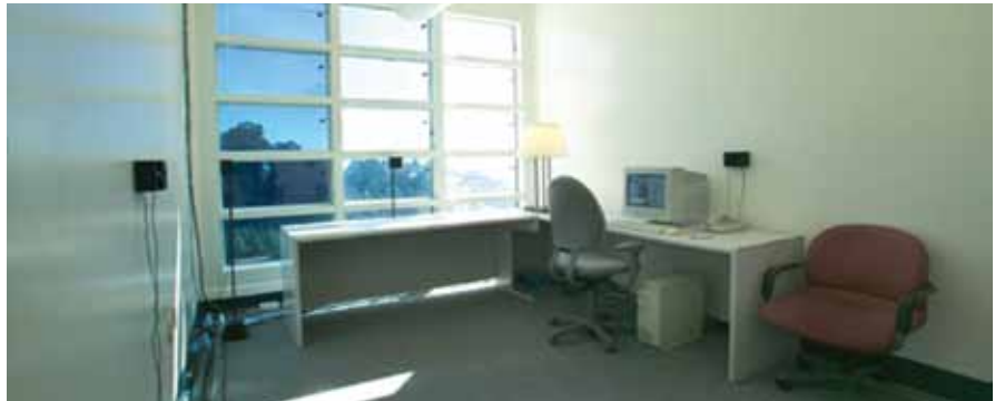
Figure 3. A photo of a façade test room with electrochromic windows configured for occupant response testing.
